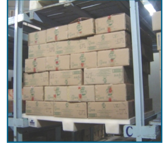
Wings On Rail for Drive-in-racking
